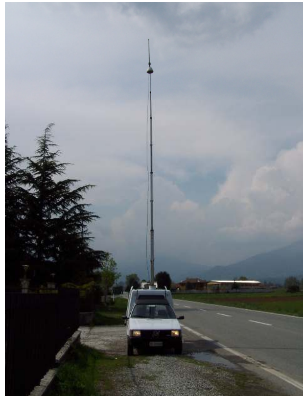
Figure 3. Equipped mobile vehicle with telescopic mast.
