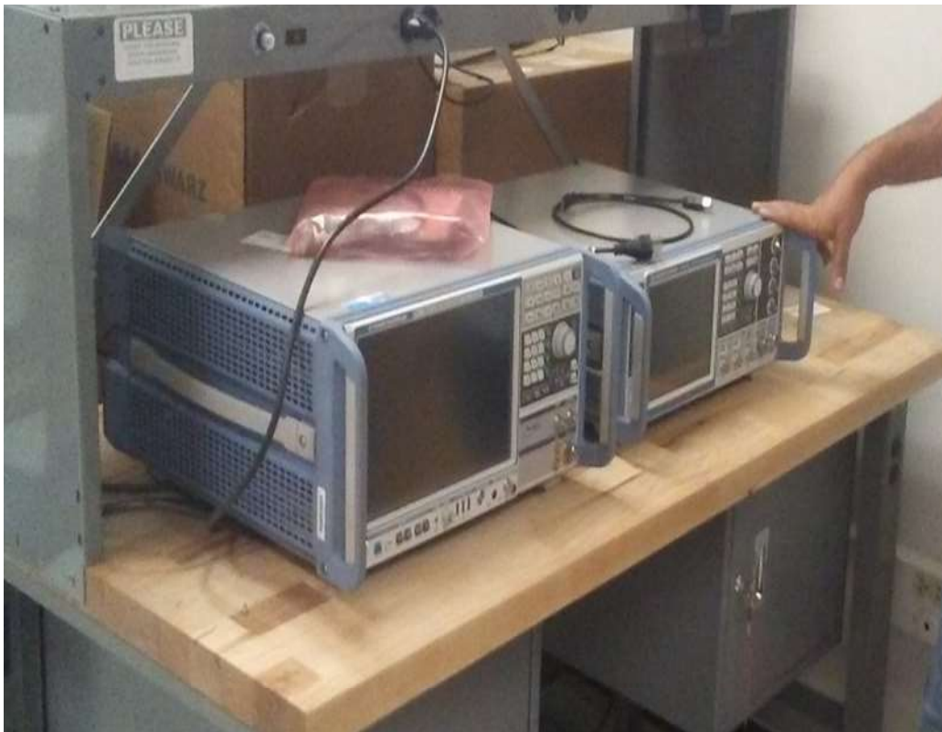
Figure A.1. Photograph of signal and spectrum analyzer (left) and vector signal generator (right).
