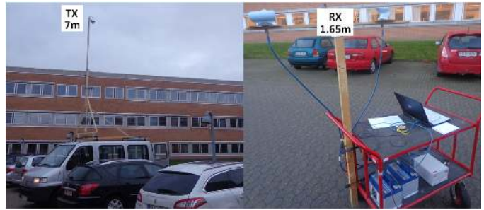
Fig. 1: Transmitter and receiver setup.
