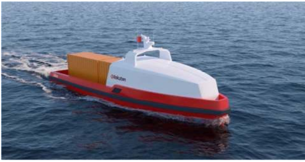
Fig. 3 USV Rakuten K22 as a result of cooperation between Maritime Robotics and Rakuten Institute of Technology
