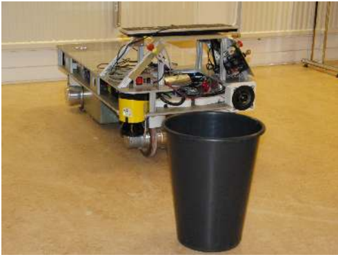
Fig. 3. The pseudo-omnidirectional mobile platform used for the experimental validation together with the basket that served as an obstacle during the experiments. The yellow laser scanner attached to the left corner of the robot was used for obstacle detection.
