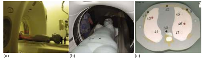
FIG. 3. Dose measurements in (a) pediatric one-year-old CIRS phantom and (b) adult female CIRS phantom. (c) The phantoms were composed of axially sliced, 25 mm thick, contiguous sections. Each section contained one or more 5 mm diameter through-holes at various organ locations.
