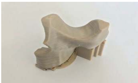
FIGURE 6: Lightweight midface-zygomatic bone PSI with support structures for immediate replacement. Thieringer FM et al. AMPA 2017.
