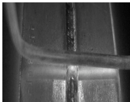
Figure 7. Principle components calculated from thermal sequences of welding line sample (e).
