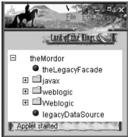
Figure 10-10: Visualization of the relevant parts of the JNDI registry of the running WebLogic 6.0 Application Server. Note the two bound references, having the lookup names theLegacyFacade and legacyDataSource .
