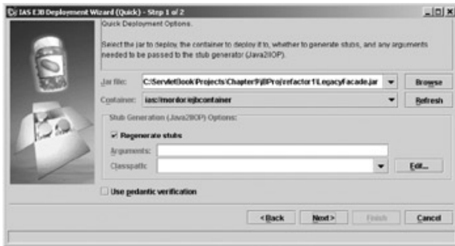
Figure 10-16: The first step of the EJB deployment wizard allows you to choose the JAR containing the bytecode files and XML configuration documents for the EJB component, as well as the EJB container where they should be deployed. Note the Regenerate stubs checkbox.
