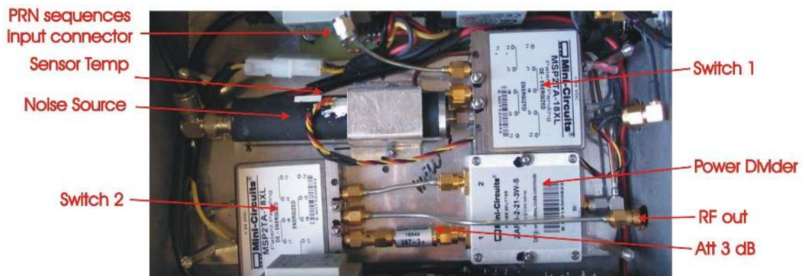
Figure 16. Hardware implementation of the selection circuitry from [6].
