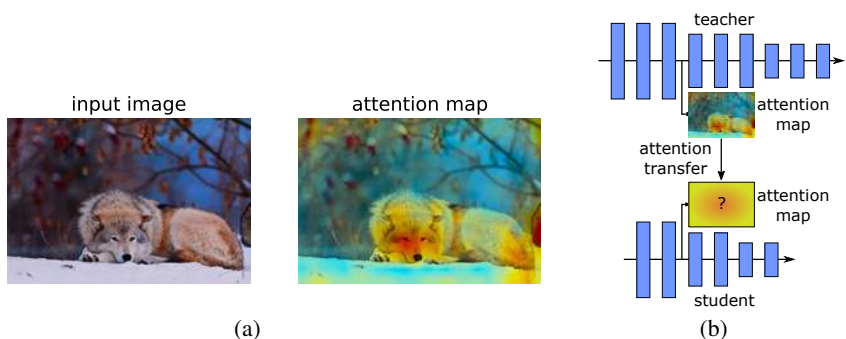
Figure 1: (a) An input image and a corresponding spatial attention map of a convolutional network that shows where the network focuses in order to classify the given image. Surely, this type of map must contain valuable information about the network. The question that we pose in this paper is the following: can we use knowledge of this type to improve the training of CNN models? (b) Schematic representation of attention transfer: a student CNN is trained so as, not only to make good predictions, but to also have similar spatial attention maps to those of an already trained teacher CNN.
