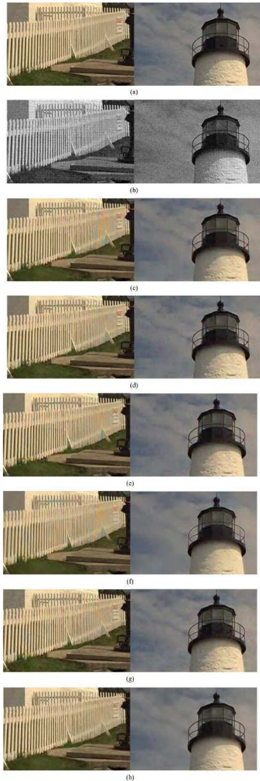
Fig. 7. Cropped images of the reconstructed color “fence” image. (a) Original image; (b) noisy CFA data ( \sigma_r = 13 , \sigma_g = 12 , \sigma_b = 10 ); (c)–(e) are reconstructed by demosaicking methods [9], [10] and [15] followed by denoising method [25]; (f) and (g) are reconstructed by joint demosaicking-denoising methods [27] and [30]; (h) is reconstructed by the proposed adaptive PCA-based CFA denoising method followed by demosaicking method [9].
