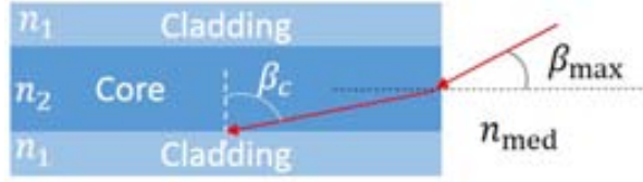
Figure 2.2: Schematic representation of an optical fibre acceptance cone.
