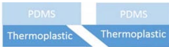
Figure 8.1: Cross section of the modular system with a thermoplastic substrate and PDMS optofluidic parts.
