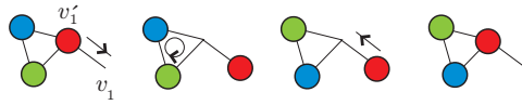
Fig. 9. With one empty vertex, pebbles on a triangle can be arranged to achieve any desired configuration. This generalizes to an arbitrary TECC.
