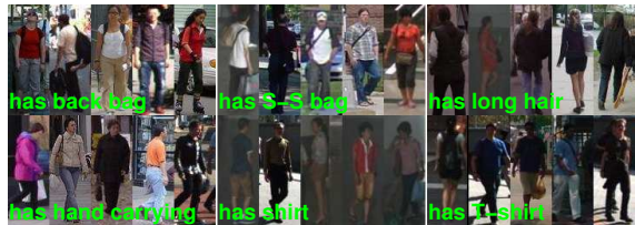
Figure 5. Some samples that are difficult to be classified in the binary attribute classification, when using AdaBoost classifiers and fusion features. Many incorrectly classified S-S bag and back bag samples have only the sash parts appearing. Results are affected by similar clothing color appearing on shoulder region ( long hair ), occlusion ( hand carrying ) and weak illumination ( shirt and T-shirt ).
