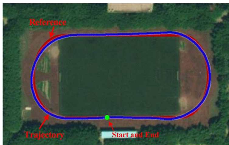
Figure 11 Walking trajectory. We choose the playground in CQUPT as the testing bed to examine the positioning accuracy of our proposed algorithm. Reference and Trajectory stand for the real trace and the tracked trace, respectively.
