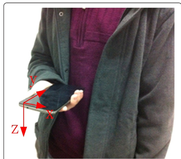
Figure 7 Hand-held smartphone during walking. The smartphone is hand-held with the X-axis in left direction, Y-axis in backward direction and Z-axis in down direction during the walking.
