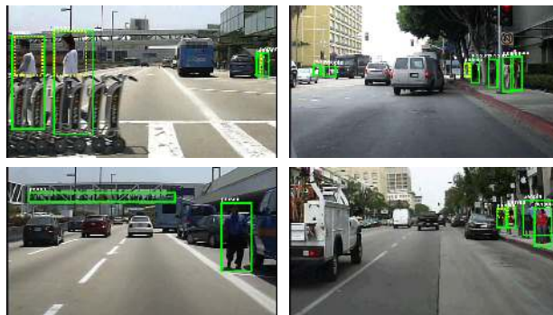
Figure 1. Example images (cropped) and annotations. The solid green boxes denote the full pedestrian extent while the dashed yellow boxes denote the visible regions. The Caltech Pedestrian Database, collected from a vehicle driving through regular traffic in an urban environment, consists of 350,000 labeled pedestrian bounding boxes in 250,000 frames.
