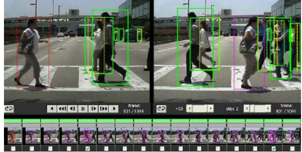
Figure 4. Screenshot of the video labeler. It is designed so that users can efficiently navigate and annotate the video with a minimum amount of labor. The most salient aspect of the labeler an interactive procedure where the user labels only a sparse set of frames and the system automatically labels intermediate frames by interpolation.
