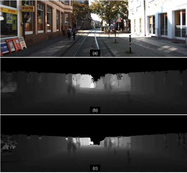
Fig. 3. (a) An example of an intensity image from KITTI database, followed by (b) a high-resolution depth image generated using the upsampling method presented in [22]. The last image, (c), was obtained using our proposed method. Visibly, Dolson’s method generates sharper depth boundaries than our proposed method, which is natural since it takes advantage of the high-resolution RGB image. It seems however to corrupt some of the depth signal, unlike our more conservative pure-depth method. For example the pedestrians near the traffic sign seem much more perceptible in (c).
