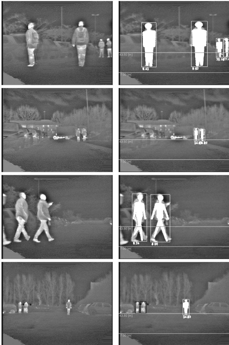
Fig. 17. Other results of pedestrian detection in different situations: with complex or simple scenarios or with one or more pedestrians. The distance (in meters) is displayed below the boxes; the two horizontal lines encode the range for which pedestrians are searched.
