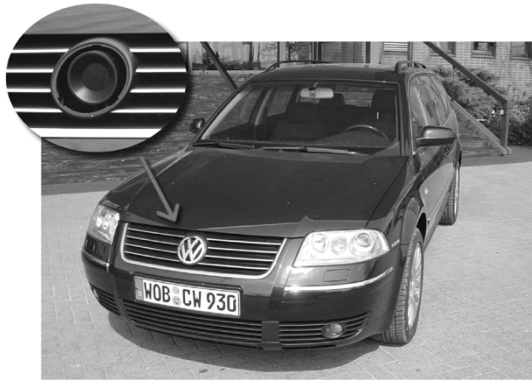
Fig. 1. The position of the infrared camera on the VW test vehicle.
