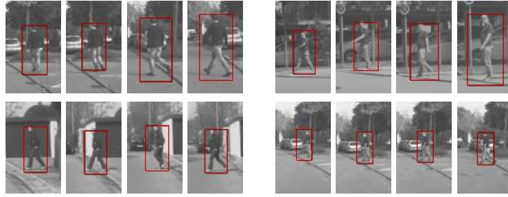
Fig. 1: Four typical pedestrian motion types: bending in (top left), stopping (top right), crossing (bottom left) and starting (bottom right) with detection bounding boxes.
