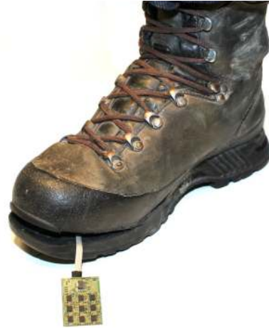
Fig. 1. Multi IMU platform pulled out from the sole of a shoe. The platform provides pedestrian tracking through ZUPT-aided inertial navigation. The measurements from the individual single-chip IMUs seen on the PCB are combined to achieve improved pedestrian tracking performance. Close-up of the platform can be found in Fig. 2 and tracking results in Fig. 3.
