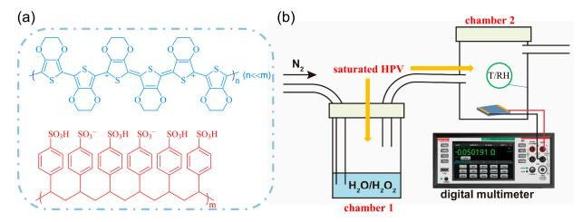
Figure 1. (a) Molecular structure of PEDOT:PSS. (b) Schematic diagram of HPV-sensing system.
