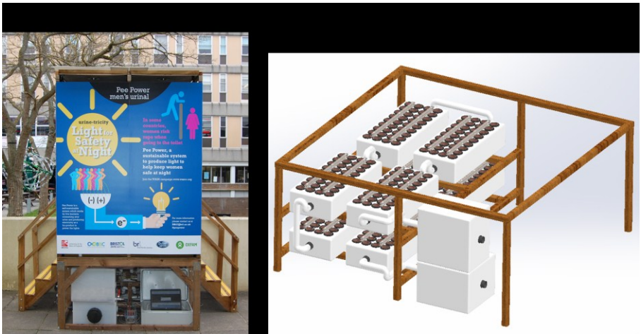
156 Figure 1. (a) Pee Power field trial funded by Oxfam at the UWE campus in February –May 157 2015; (b) 3D representation of the MFC stack with the inlet and outlet tanks underneath the 158 urinal. 159
