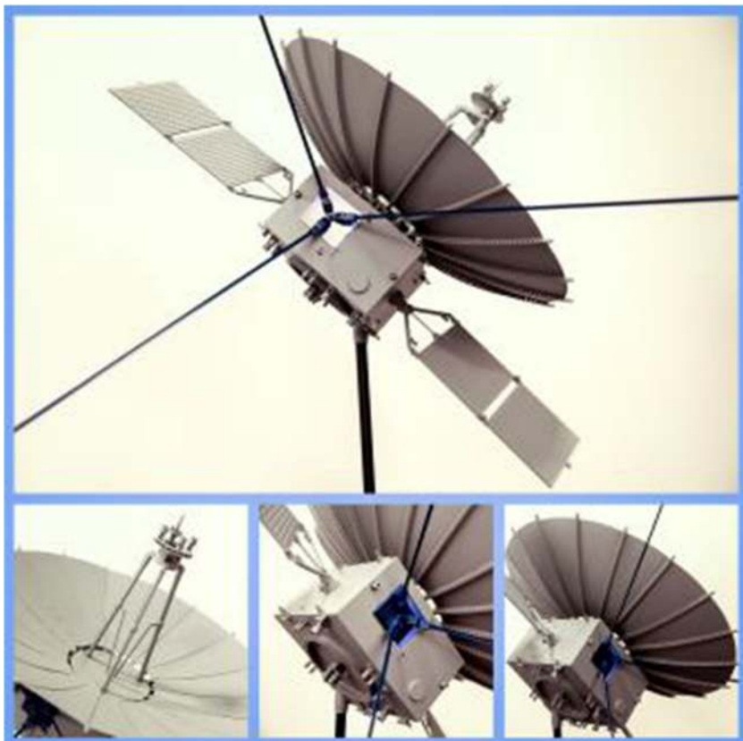
Fig. 6 Rendered view of NCLE, the tripole attached to the Chang-e'4 relay satellite
