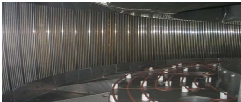
Fig. 6. The 200\ ^3\text{He} position sensitive detectors are installed inside the detector chamber.
