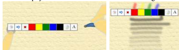
Fig. 8. Left: Dragging from the Finger Shadow (here with the pen) opens the menu. Right: Finger painting using the color pots.
