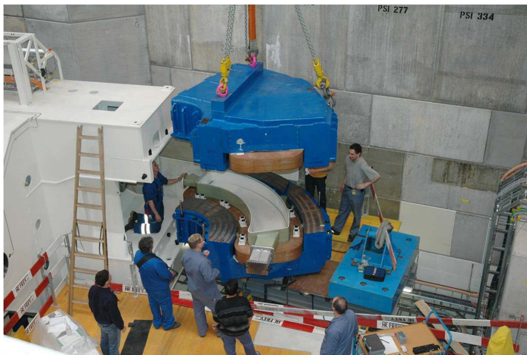
Fig. 12. Photograph of the 90° bending magnet being mounted on the Gantry 2. A very interesting detail is the integrated vacuum chamber embracing the poles of the magnet.
