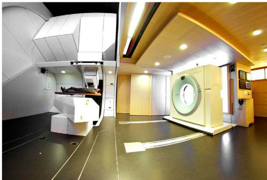
Fig. 3. The layout of the Gantry 2 room with patient table, nozzle and the sliding CT (a fish eye photograph).
