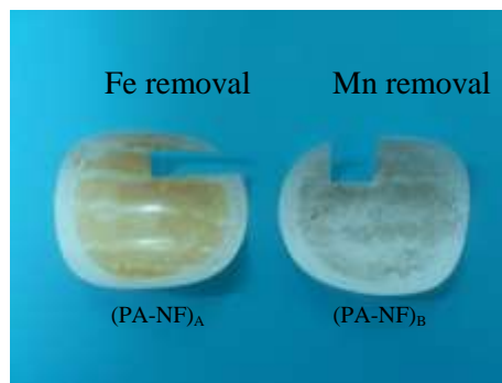
Figure 4. Visualization on physical quality of fouled PA-NF membranes for filtration at 5 bar and pH 9
