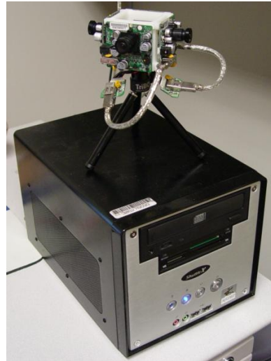
Fig. 1. The complete CAMEO system consists of several calibrated firewire cameras and a portable image-processing workstation.
