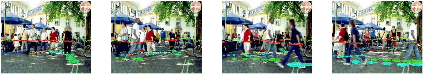
Fig. 7. Four images of the outdoor experiments carried out in the inner city of Freiburg. The information of the laser range finder and the tracking system were projected onto a recorded video sequence. The images from left to right show the tracking results at timesteps t = 335, 353, 365 and 381 . Laser range measurements are shown as small green dots (background) or small red dots (detected pedestrians). The traces of the observed pedestrians are drawn with colored ellipses.
