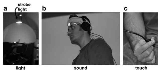
Fig. 2 Apparatus. a Participants sat inside a plastic hemisphere. A strobe light was mounted pointing downwards to provide a diffuse flash of light as required. b Participants wore headphones for presentation of sound stimuli. c Participants held a vibrotactile stimulator between their thumb and index finger for presentation of touch stimuli
