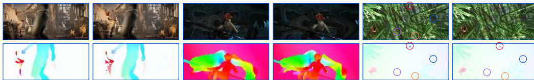
Figure 8: Qualitative examples of optical flow. For each image pair, we show the two frames (top), and then the estimated flow (bottom left) and the ground-truth flow (bottom right). In the left example, we see one person under heavy occlusion where the correct flow is propagated into a region with few details. Another person in the foreground has clothes with little texture and substantial blur, and yet the algorithm can propagate the flow across the entire region. In the center example, we see very large motions from both the dragon and the person, yet many fine structures are preserved like the pole. On the right, we see a forest scene with a few extremely small objects with very subtle motions (circled) which our algorithm is able to detect and segment correctly.
