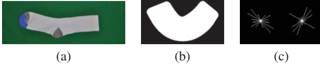
Fig. 5. We extract the local shape by using a HOG representation. (a) An image of a sock. The blue region indicates a segment along the contour. (b) A mask of a segment along the contour is computed, and rotated such that it is upright. (c) For each segment mask, gradient information is binned into local 9 dimensional orientation histograms. Each bin is visualized with small line segments that have a length according to the accumulated gradient strength.
