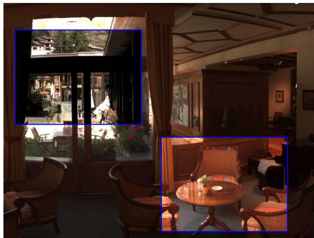
Figure 8: CAFETERIA sequence, dynamic range -1.9 \div 3.6[\log cd/m^2] . The background frame is clamped to a displayable range. Our dynamic range exploration tool, visible as two windows, shows a luminance range -1.0 \div 1.0[\log cd/m^2] (lower right) and a high luminance range 1.0 \div 3.0[\log cd/m^2] (upper left). Details in these windows are not visible in LDR video. The source panorama courtesy of Spheron, Inc.
