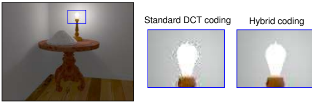
Figure 5: Quality comparison of the standard DCT coding of the block and our hybrid frequency and luminance space coding. Quantized DCT blocks show artifacts at sharp edges, which are not visible for the hybrid encoding. The hybrid encoding increased size of the bit-stream by 7%.
