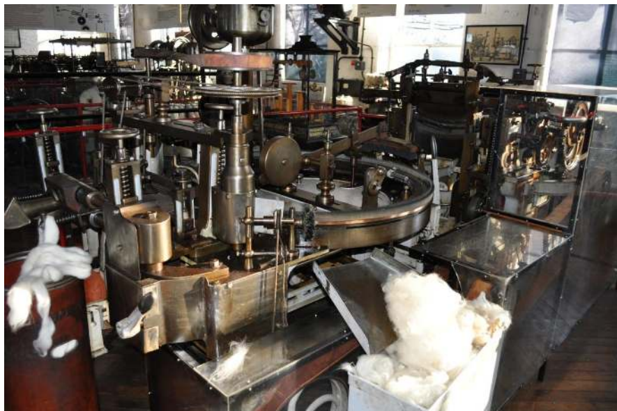
Picture 3-9: The Lister Comb patented in 1849 by Samuel C. Lister of Manningham was one of several local inventions that gave Bradford an edge in woolen manufacturing. Combing straightens the wool fibers, separating the short wool from the long wool (Reid, 2010)
