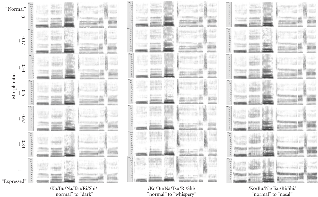
FIGURE 2: Spectrograms of synthesized voices with morphing ratios from 0 to 1.
