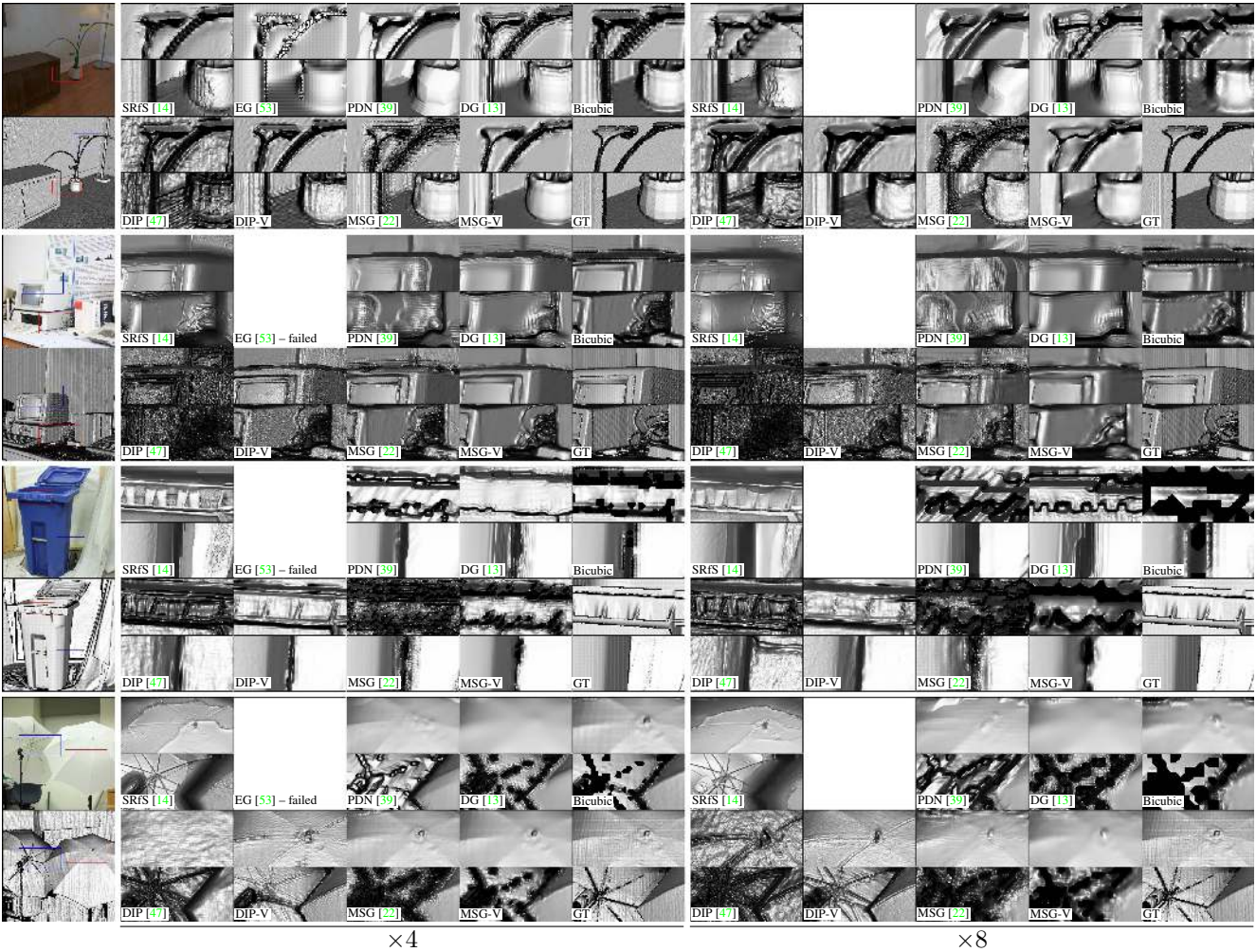
Figure 6: Depth map renderings corresponding to super-resolution results on “Plant” from “ICL-NUIM” and “Vintage”, “Recycle” and “Umbrella” from Middlebury datasets with the scaling factor of 4 on the left and the scaling factor of 8 on the right. Best viewed in large scale.
