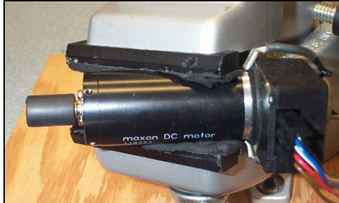
Figure 1: Haptic display and experiment setup. A brass knob mounted directly on the motor shaft was covered with 1-mm rubber to prevent slipping while adding little compliance. The adjustable vise mount and cushioned armrest made the setup customizable and comfortable. Participants were asked to hold the knob lightly between thumb and index finger.
