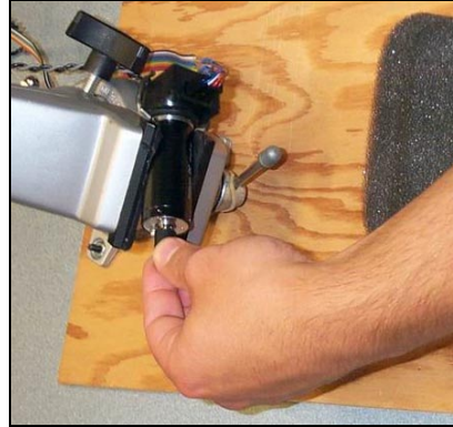
Figure 1: Haptic display and experiment setup. A brass knob mounted directly on the motor shaft was covered with 1-mm rubber to prevent slipping while adding little compliance. The adjustable vise mount and cushioned armrest made the setup customizable and comfortable. Participants were asked to hold the knob lightly between thumb and index finger.
