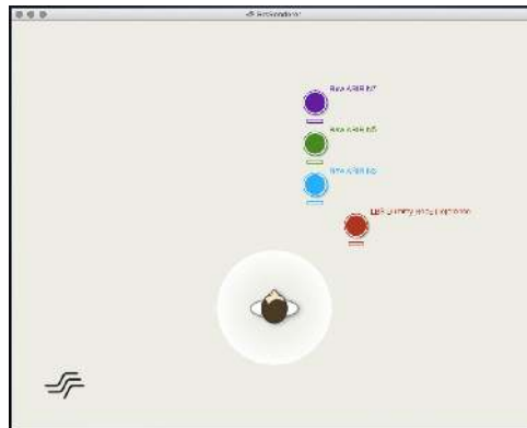
Figure 3.2: The graphical user interface of the SoundScape Renderer in the Binaural Room Synthesis (BRS) mode shows an example scene consisting of four sound sources. Every sound source represents one BRIR set loaded into the working memory. Every BRIR set can be unmuted dynamically which enables the real-time rendering of a dynamic binaural synthesis.
