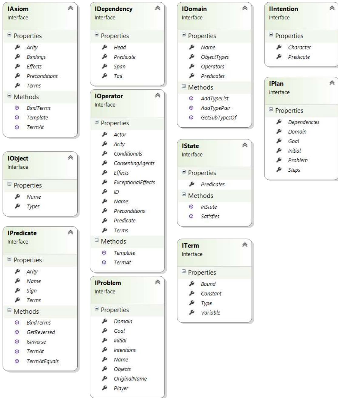
Figure 5.2: Diagram of interfaces for GME's PDDL data structures. The diagram is generated by Microsoft Visual Studio 2015. GME models axioms, dependencies, domains, intentions, objects, operators, plans, predicates, problems, states, and terms. When implemented, these interfaces form the basic building blocks from which interactive narrative trees are constructed.
