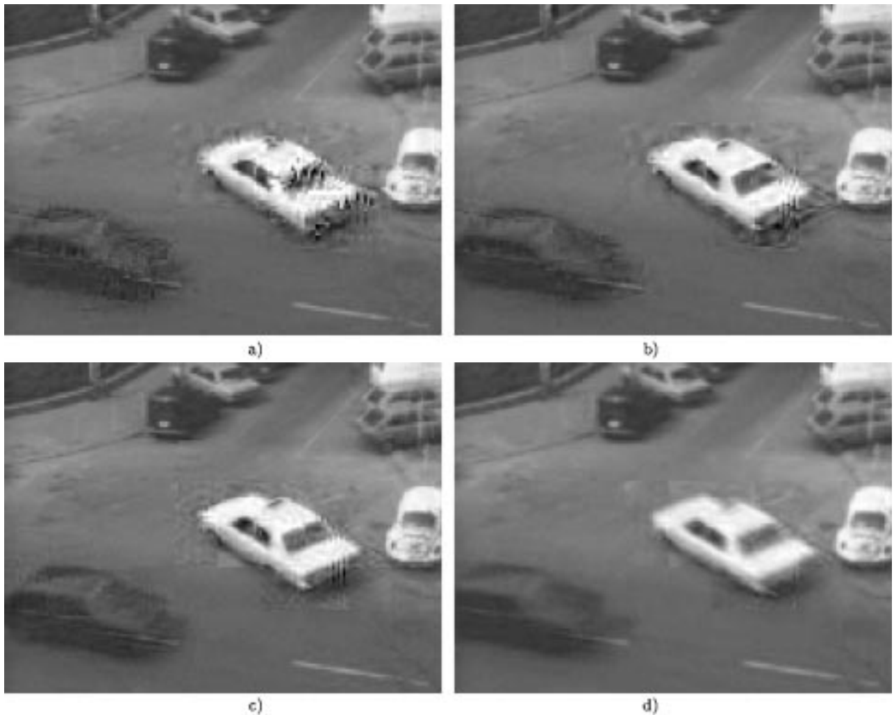
Fig. 15. Reconstruction results with the Taxi sequence using previously reported encoding configurations (a-b) and the proposed 2-D or 3-D alternatives (c-d). (a) Fixed size BMA for motion estimation and MPEG-like quantization (linear MPE). (b) Unweighted variable-size BMA and MPEG-like quantization (linear MPE). (c) Perceptually weighted variable-size BMA and 2-D nonlinear MPE quantization. (d) Perceptually weighted variable-size BMA and 2-D nonlinear MPE quantization and temporal filtering.
