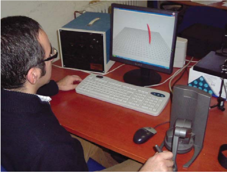
Figure 1. Subject touching a virtual surface through a stylus-like device.
