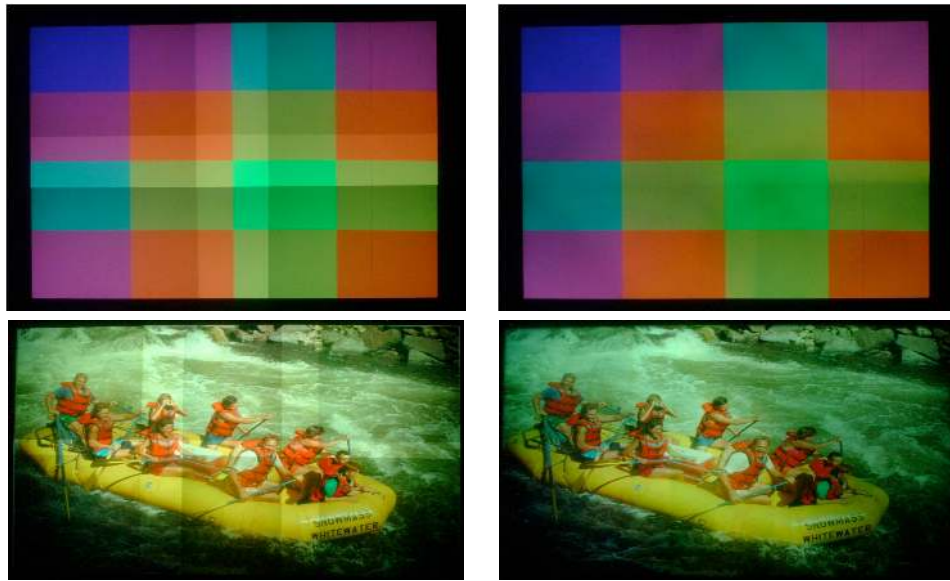
Fig. 12. Digital photographs of displays made of 2 \times 2 and 2 \times 3 array of four ( 1.5' \times 2.5' in size) and six ( 3' \times 4' in size) projectors of respectively. Left: Before correction. Right: After constrained gradient based luminance smoothing. Note that we are able to achieve perceptual seamlessness even for flat colors (top), the most critical test image for our algorithm.
