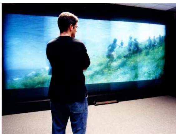
Fig. 14. The correction applied to a non-Lambertian screen and viewed from a view direction that makes an angle of less than 20 degrees with the screen.
