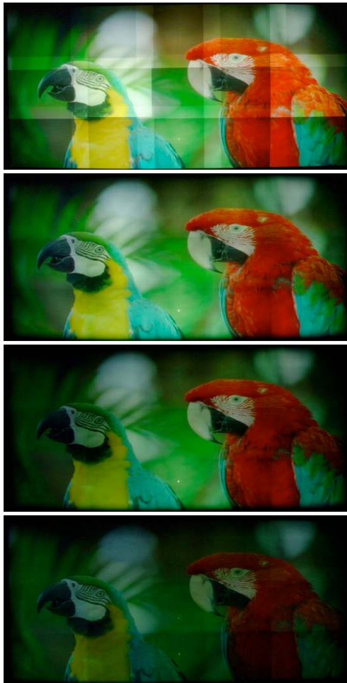
Fig. 10. Digital photographs of a fifteen projector tiled display ( 8' \times 10' in size) before any correction (top), after constraint gradient based smoothing with smoothing parameter of \lambda = 400 , (second from top) \lambda = 800 (third from top) and after photometric uniformity i.e. \lambda = \infty (bottom). Note that the dynamic range of the display reduces as the smoothing parameter increases. At \lambda = \infty is the special case of photometric uniformity where the display has a very low dynamic range.
