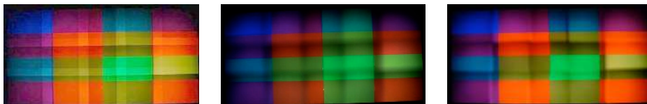
Fig. 13. The fifteen projector tiled display before blending (left), after software blending (middle), and after optical blending using physical mask (right).
