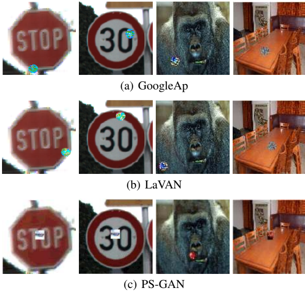
Figure 4: Adversarial patches generated by GoogleAp, LaVAN and PS-GAN on GTSRB and ImageNet in the semi-whitebox setting. All the attacked images are misclassified.
