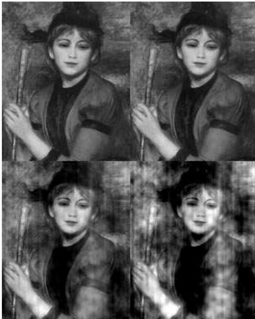
Figure 2. Example of DCT-spread spectrum technique in [46]; from left to right, top to bottom: original, a = 0.1 , a = 0.5 , a = 1.0
