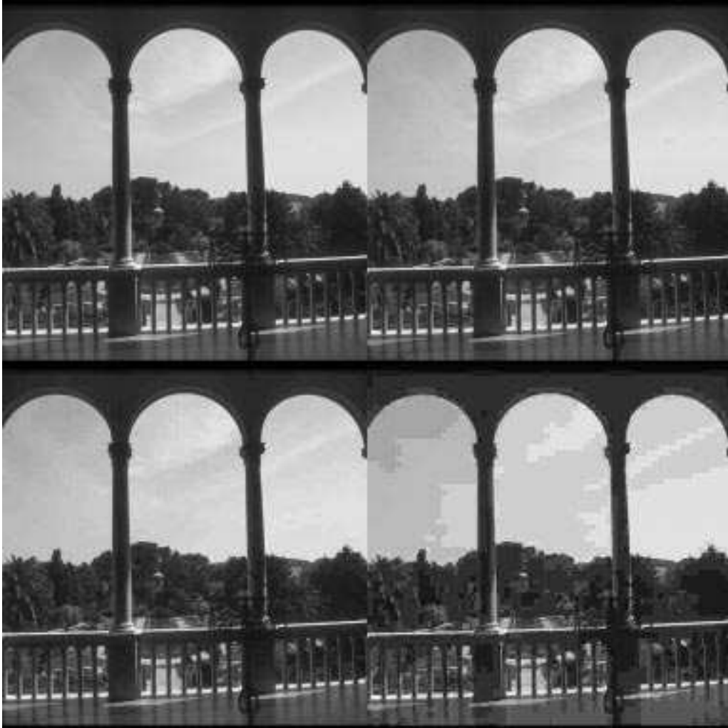
Figure 7. Uncompressed and JPEG compressed versions of the marked garden image From left to right, top to bottom: uncompressed image, bpp = 0.6, 0.4 and 0.18
