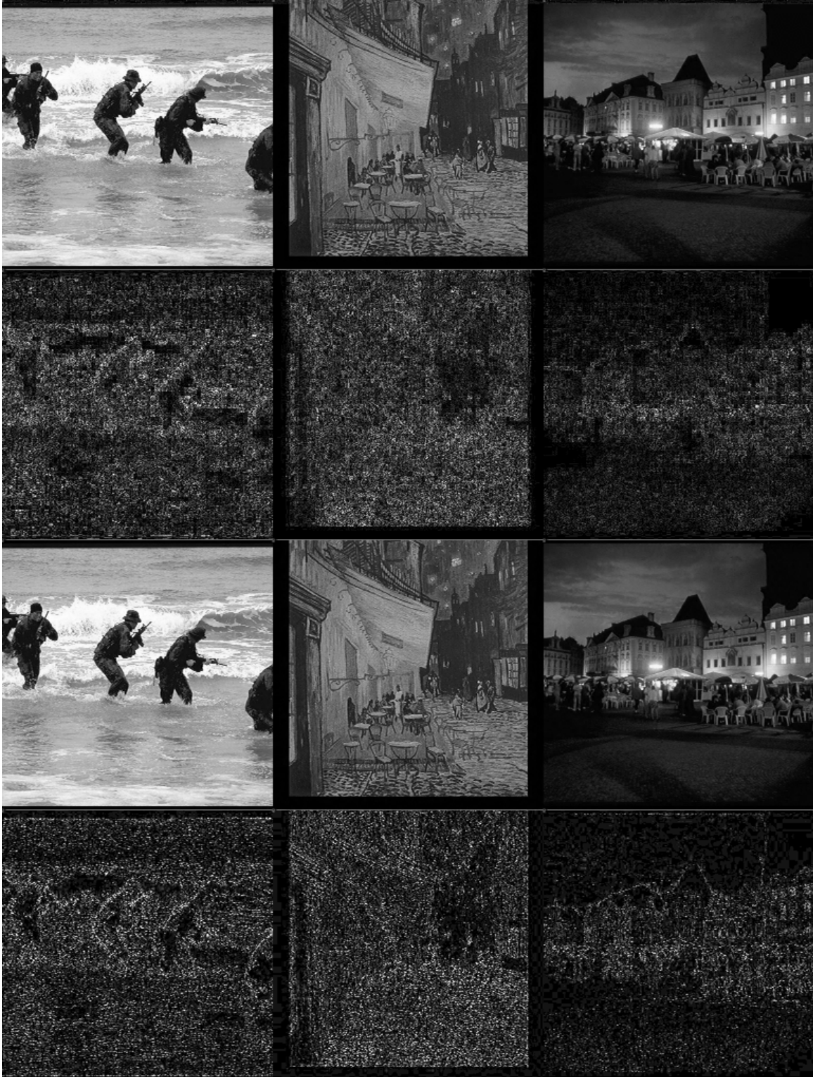
Figure 5. IA-DCT watermarked images (top row), IA-W watermarked images (third row) with corresponding IA-DCT watermarks (second row) and IA-W watermarks (fourth row)
