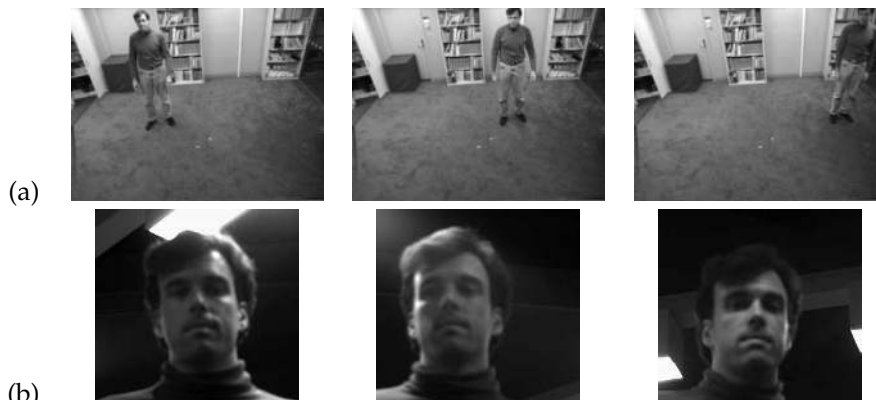
Figure 3: Images acquired from wide (a) and narrow (b) field of view cameras as user moved across room and narrow camera tracks head.
