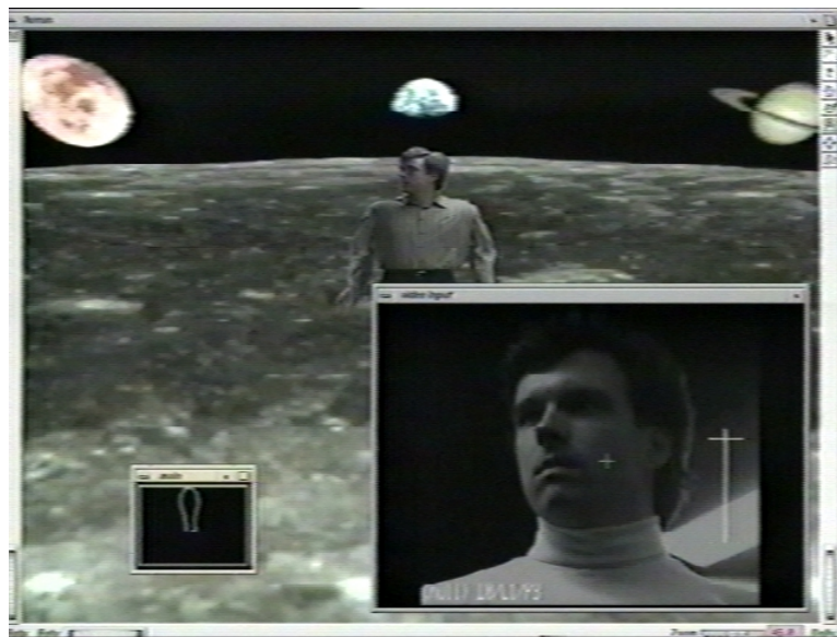
Figure 13: Avatar driven by multiple scales of visual tracking; subwindows show silhouette from coarse-scale figure/ground segmentation and fine scale face pose analysis on active camera imagery.
