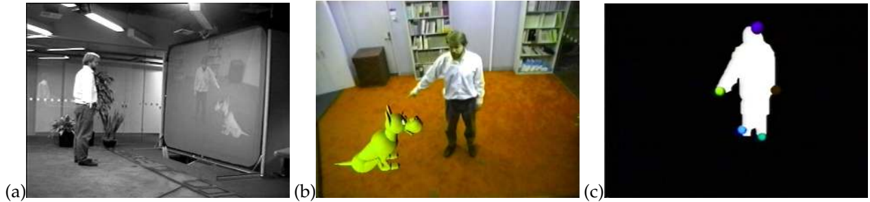
Figure 2: Coarse-scale person tracking in a system for vision-based interaction with a virtual environment. (a) A user sees himself in a “magic mirror”, composited in a virtual environment. Computer vision routines analyze the image of the person to allow him to effect the virtual world through direct manipulation and/or gestural commands. (b) Image presented on video wall. With this system, user can interact with virtual agents, such as the dog character in our ALIVE system [12, 6] (c) Results of feature tracking routine; head, hands, and feet are marked with color-coded balls.
