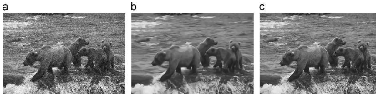
Fig. 4. Accurate noise variance as input to the algorithm in [40] produces poorer quality denoised images: (a) noisy image ( \sigma = 0.0158 , MS\text{-}SSIM_D = 107.26 ), (b) denoised with \sigma = 0.0158 ( MS\text{-}SSIM_D = 64.00 ) and (c) denoised with \sigma = 0.0040 ( MS\text{-}SSIM_D = 53.82 ).
