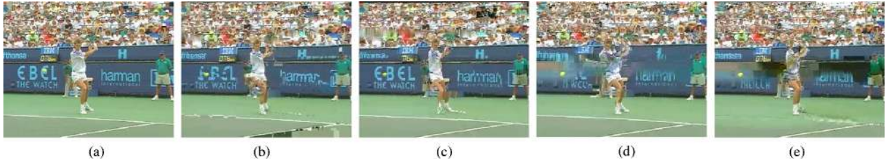
Fig. 13. Subjective quality comparison on the 15th frame of the Stefan test video clip ( P_B = 5\% ). (a) Original video clip. (b) FEC-FL(0). (c) FEC-FL(8). (d) GRIP. (e) Equal FEC.
