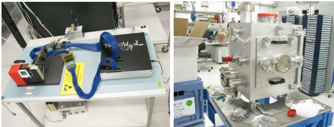
FIGURE 3. Picture of the “naked” P2M system, used for in-air lab tests (left) and of the vacuum vessel (right) developed for sub-zero operation and low-energy-photon detection
