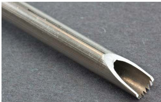
Fig. 6. Photograph with a view of the teeth of the decorticator tool.
